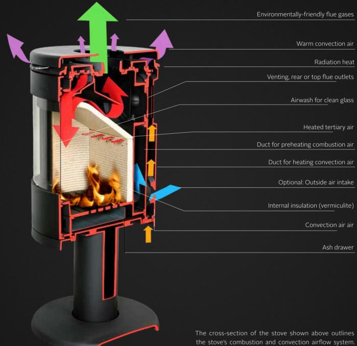
the stove's combustion and convection airflow system. Cold air is drawn into the stove and heated as its passes through the cast iron channels (the heated air washes the glass keeping it clean, clear and free from soot). The hot air also provides perfectly heated combustion air
