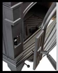
Cast iron door features a raised, pinched door seal and secure locking door handle that ensures an air-tight seal around the glass, so the door will never warp or flex. The frame also protects the glass gasket from direct contact with the fire.
